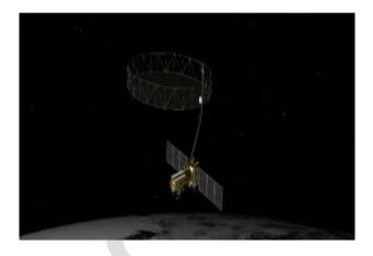
Technological Highlights First satellite to use dual-frequency Synthetic Aperture Radar (SAR): L-band (NASA) S-band (ISRO) Uses NASA's 12-metre unfurlable mesh reflector antenna Integrates with ISRO's modified I3K satellite bus
