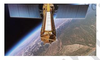
Synthetic Aperture Radar (SAR) is a form of radar that uses the motion of a radar antenna to create high-resolution images of the Earth's surface. It achieves this by transmitting microwave pulses and analysing the returning echoes, effectively simulating a much larger antenna than the physical one on the moving platform.
