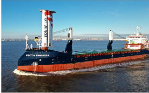
Wind in sails: The Vectis Progress, a cargo ship with an experimental sail, AirWing, on the River Humber after leaving port in Kingston Hull in England. The advanced technology sail is a wind propulsion system comprising novel AirFlow technology to maximise thrust a savings. Airwing has embarked on its first journey using wind power to propel a cargo ship from England to Canada to cut emissions.
