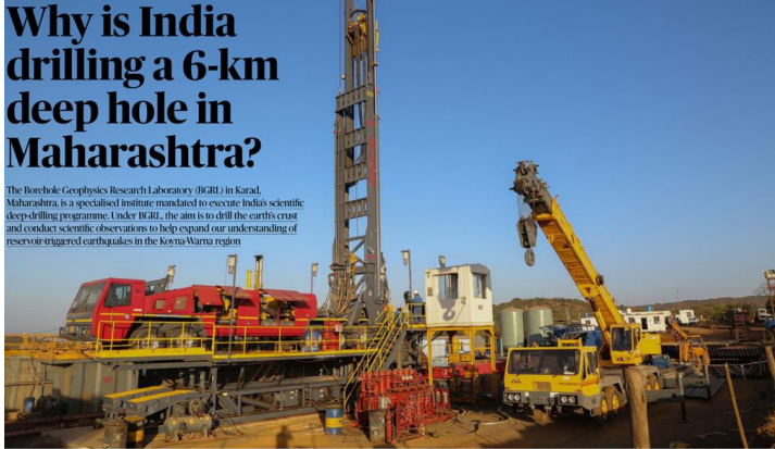
PHOTO: At the deep drilling site in Koyana region, Maharashtra, the towering drilling rig is seen surrounded by associated equipment, an on-site mud logging unit, gas analysis lab, and a geological studies lab. MSR, KSL
