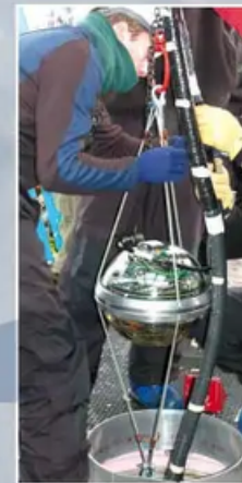
Light sensors 80 strings holding 60 sensors each are lowered into the holes. This has to be done quickly before the water in the hole refreezes
