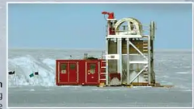
Hot water station Used for drilling holes in the ice
